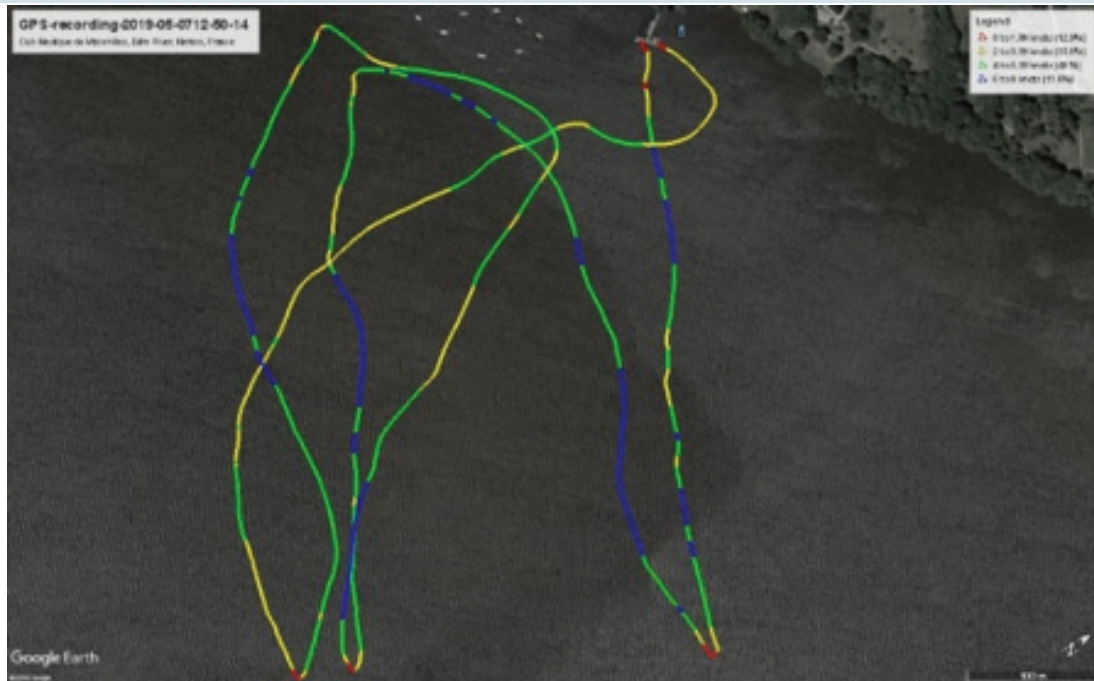
Figure 12. Example of ship trajectory and speed measured during the trial. The colors indicate the speed of the sailing ship. Background and map image using Google Earth.
