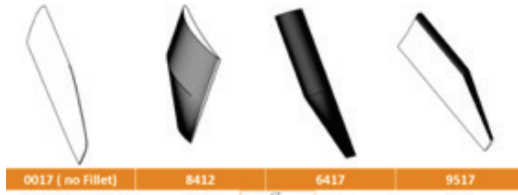
Figure 9. CAD Design for NACA 0017 and Expected Deformed Shape NACA 8412, 6417 and 9517.
