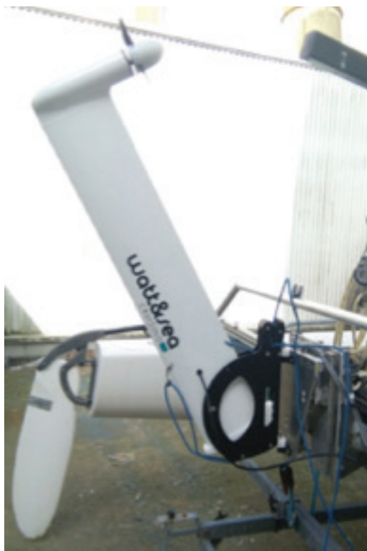
Figure 5. Watt & Sea cruising 600 hydrogenerator.
