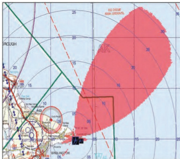
Figure 7. Coverage area of the GPS jamming unit at 25m above ground level on maximum power of 1.58W ERP. (Grant, Williams, Ward, & Basker, 2008 - Image courtesy of DSTL).
