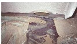
**Figure 3.** Sediments accumulate in ballast water tanks in areas with flow stagnation.
